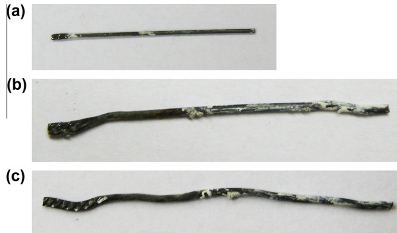
Fig. 12. (a) straight fibres, (b) hooked-end fibres, (c) undulated fibres, after pullout test.
